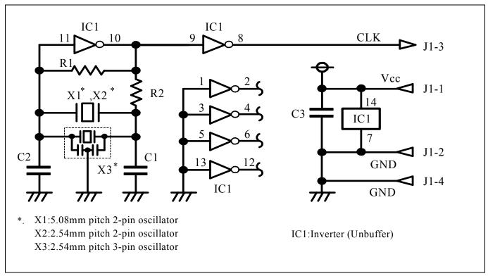
Figure 2.21 Circuits of the oscillator circuit bare board OSC-2
